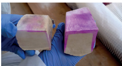
The depth of penetration of the nanolime was gauged with the use of phenolphthalein, which turns pink in the presence of un-carbonated lime. The sample of stone treated with the nanolime was cut in half and sprayed with the indicator: the depth of penetration is clearly seen.
